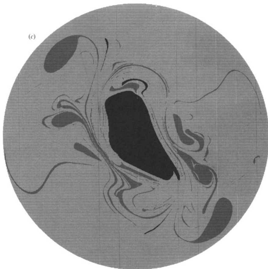
FIGURE 7. The nonlinear development of an unstable band lying between \theta_{0s} = 10^\circ and \theta_{0n} = 20^\circ , in the presence of two finite polar vortices of oppositely signed circulation ( \theta_{np} = 50^\circ and \theta_{sp} = -40^\circ ). The vorticity jump into the band \tilde{\omega}_b = \frac{1}{2} is half of that across the edges of the polar vortices. (a) Orthographic view from \theta = 20^\circ , \phi = 20^\circ . (b) Polar stereographic view (the outer disc is at \theta = -20^\circ ). (c) Enlargement of the view in (b) at t = 49 .
